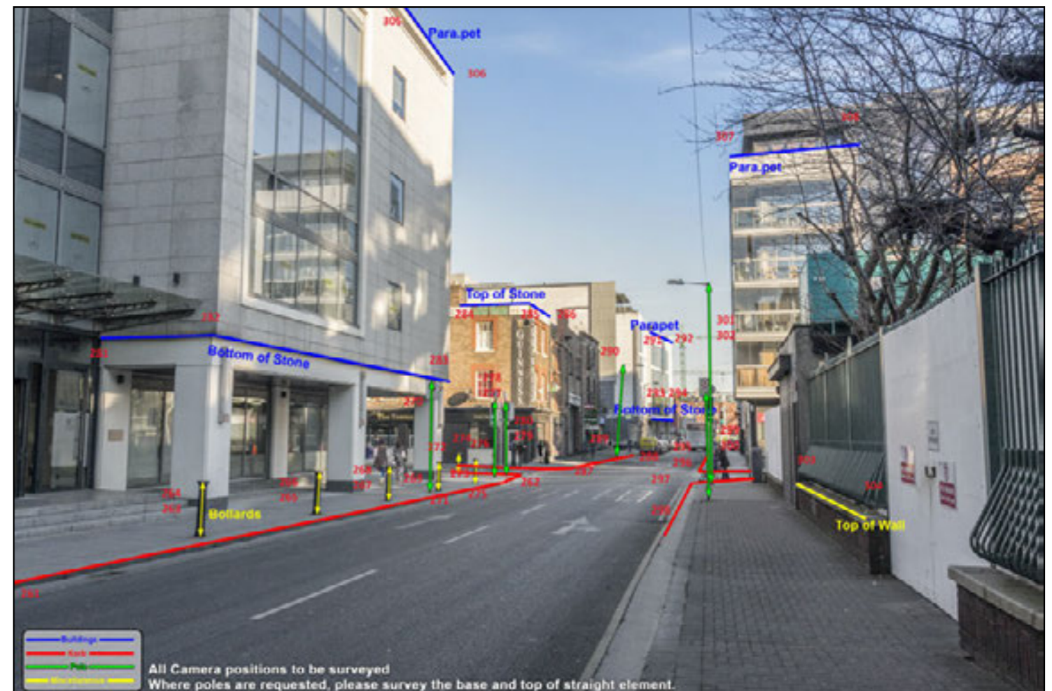
Fig.8: Fixed reference points fully surveyed and numbered.
